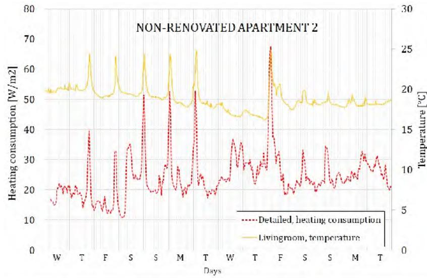
Figure 4.4: Graph of temperature and heating consumption for Non-renovated Apartment 2
