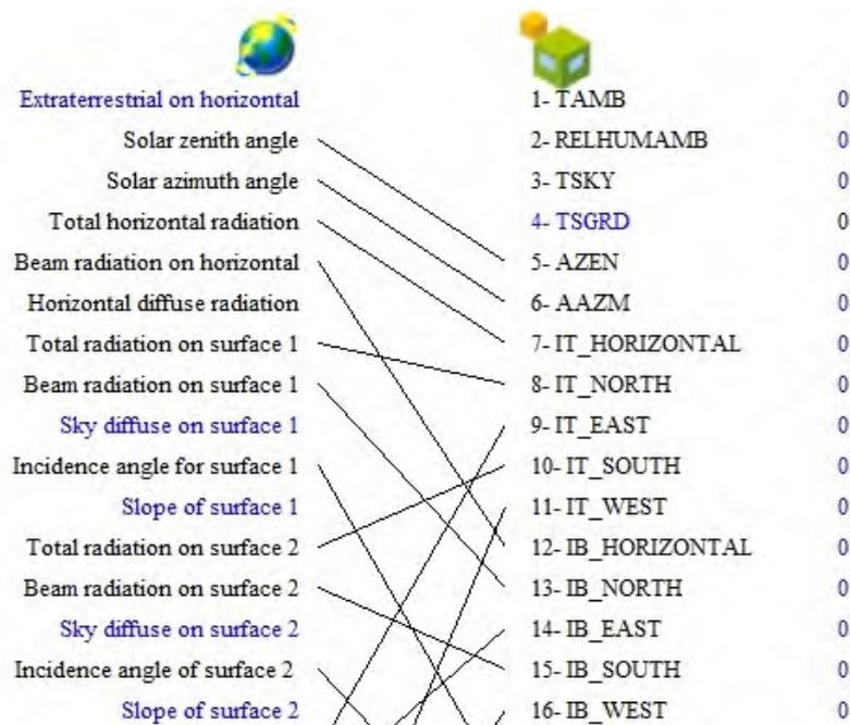
Figure 3.6: Definition of connection between Type16c and Type56a
