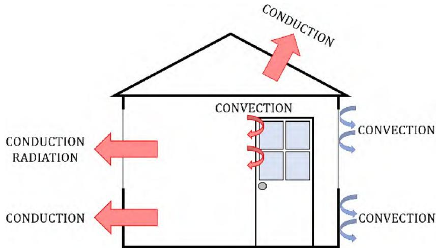
Figure 2.1: Heat transfer modes through a building envelope
