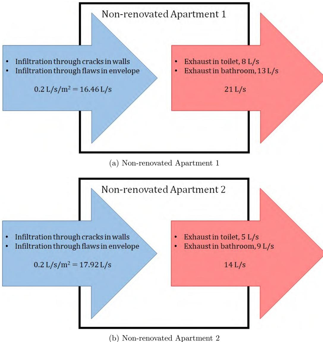
Figure 3.2: Air balance for the non-renovated apartments
