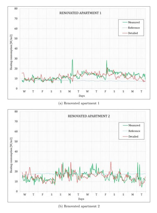
Figure 4.1: Comparison of heating consumption for renovated apartments
