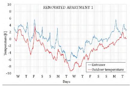
Figure 4.9: Graph comparing outdoor and Entrance temperature at Renovated Apartment 1
