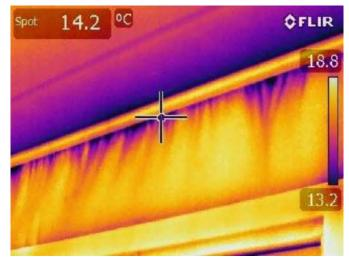
Figure 4.8: Thermographic photo of joint at facade/ceiling at Renovated Apartment 1 Entrance
