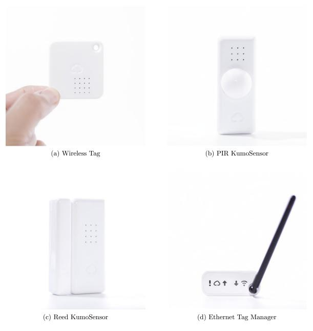
Figure 2.5: The sensors used from the Wireless Sensor Tag System [4]
