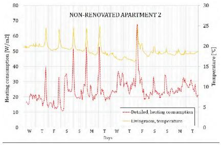
Figure 4.4: Graph of temperature and heating consumption for Non-renovated Apartment 2
